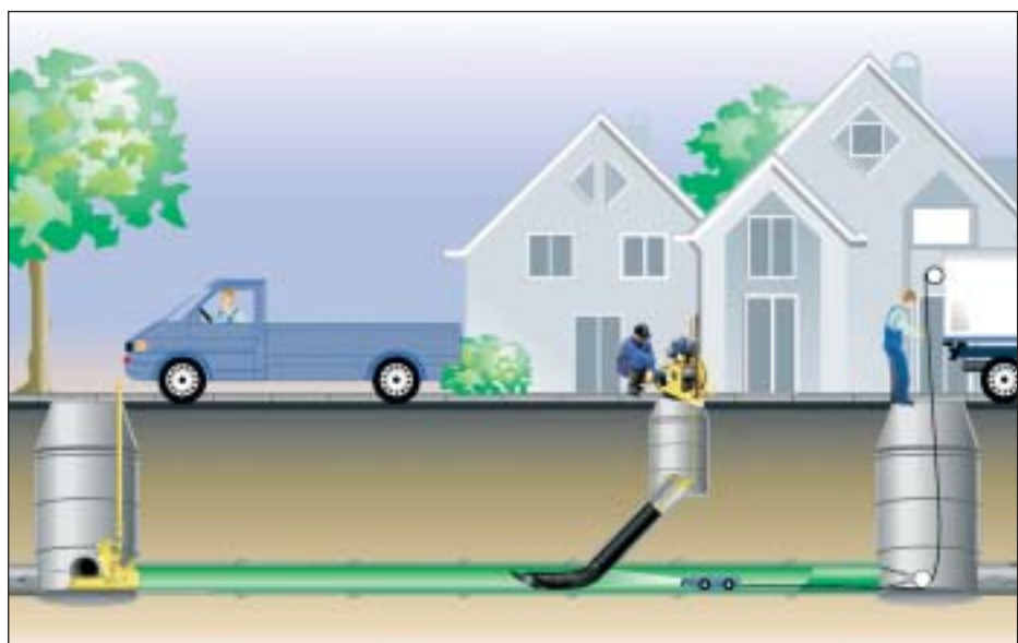
Close-fit lining and subsequent lateral installation.
